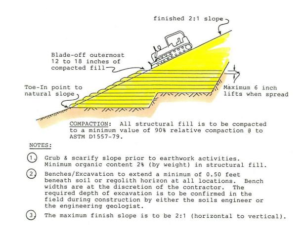
Trimming involves drifting of the upper 1.5 feet by a tracked dozer, removing loose material. Unfortunately, it is much more difficult to plant a trimmed slope, and "tree pits" may be required to plant bushes or trees so that their roots can tap successfully.
