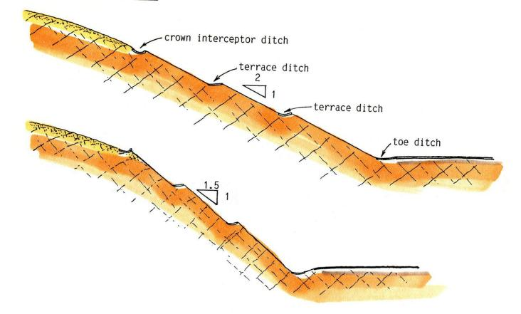
Benched cuts with drainage interceptor terraces became commonplace with the Interstate Highway program in the mid-1950s
