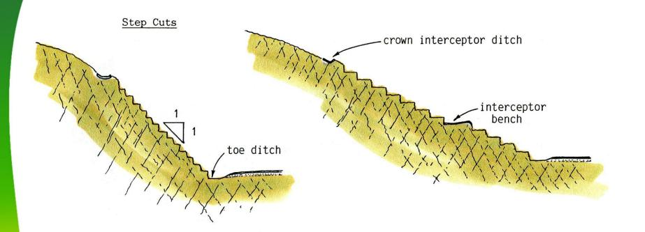
The Bureau of Public Roads introduced 1:1 step cuts in Arizona in the late 1920s. They have since been applied to slopes as flat as 2:1, as shown at right. A drainage interceptor bench must be inclined to provide gravity flow for drainage
